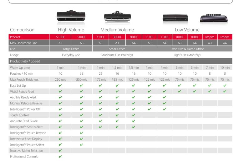
Notes: All timings shown are approximate. On A3 machines laminating speed can be increased by up to 30% by using GBC HighSpeed<sup>TM</sup> Pouches (see page 30).
