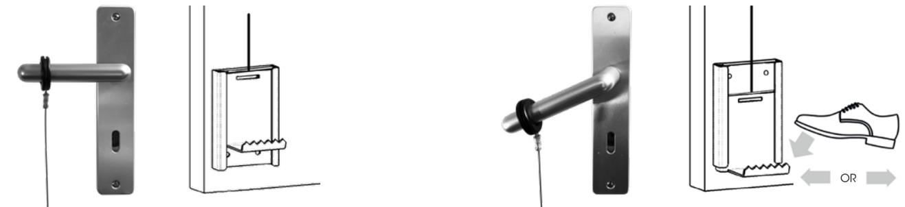
Door closed – handle in horizontal position, sliding plate in the upper position
