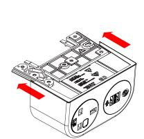
3. Slide PHASE onto the bracket until the clips engage.
