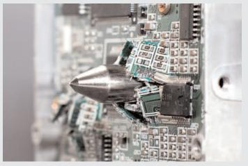
The high quality punching die is made of hardened, nickelplated tool steel. Durability is also guaranteed by a powerful single phase motor rated for continuous operation in combination with the sturdy "twin drive system".
