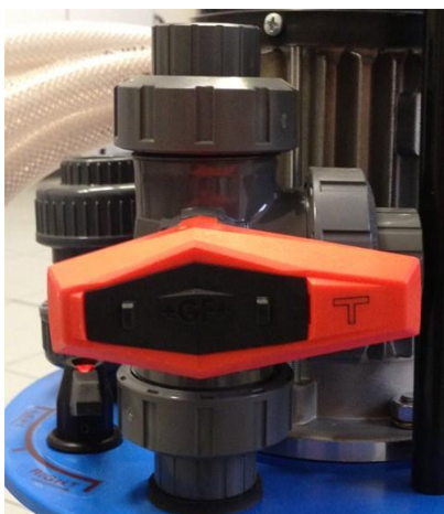
Valve in dump position
