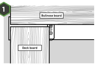
Insert the Universal Clip as shown in the diagram with the front of the clip positioned in the groove of the secured bullnose deck board.
