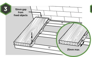
To secure the first board, use one Universal Clip and screw on every joist. Take a screw, place in the hole located in the Universal Clip and screw into the wooden joist. **Do not tighten at this stage.** Make sure the boards do not overhang the joist at the edge by **more than 25mm** and a **10mm expansion gap** should be left between the wall or other fixed objects surrounding the deck.
